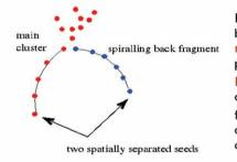
For terminating hit "i" of spiraling back fragment candidate (# hits < nMergeSpiral), calculate merging parameter w.r.t. nearest hits "j" ( $r_{ij}$  < RCut) belonging to high multiplicity clusters. If min( $s_{ij}$ ) < sCut, merge fragment candidate to the corresponding high multiplicity cluster
