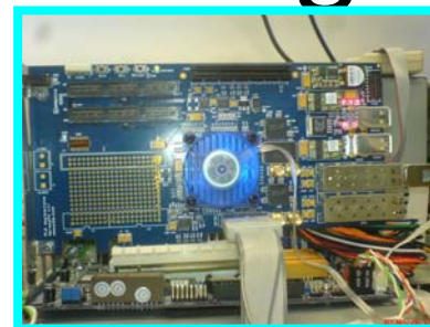
working FPGA based Ethernet system, using RAW frames
