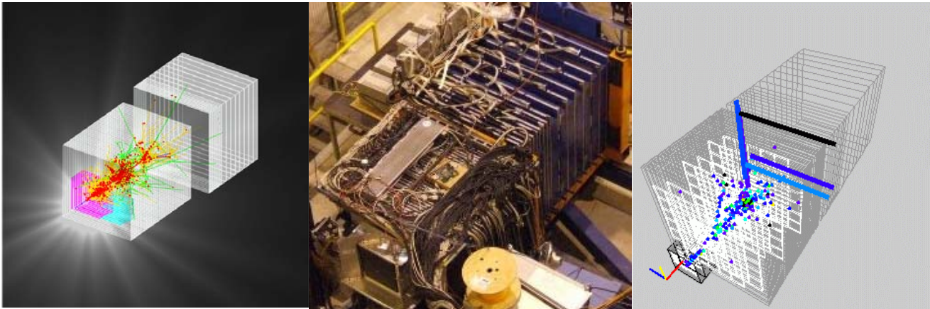
Figure 3.1: The experiment from concept to reality. A simulated hadron event in the combined testbeam setup (left). The installation of the three calorimeters at CERN (centre). One of the data events taken in 2006 (right).
