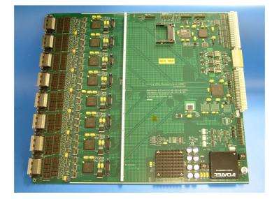
Figure 1: Prototype VME readout board.
