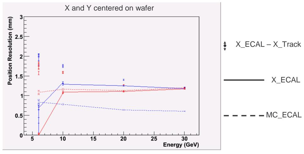
Y is even better than MC, and fail only at 6 GeV where MS has to be considered X is better than 06 data but still 0.5 mm worse than MC
