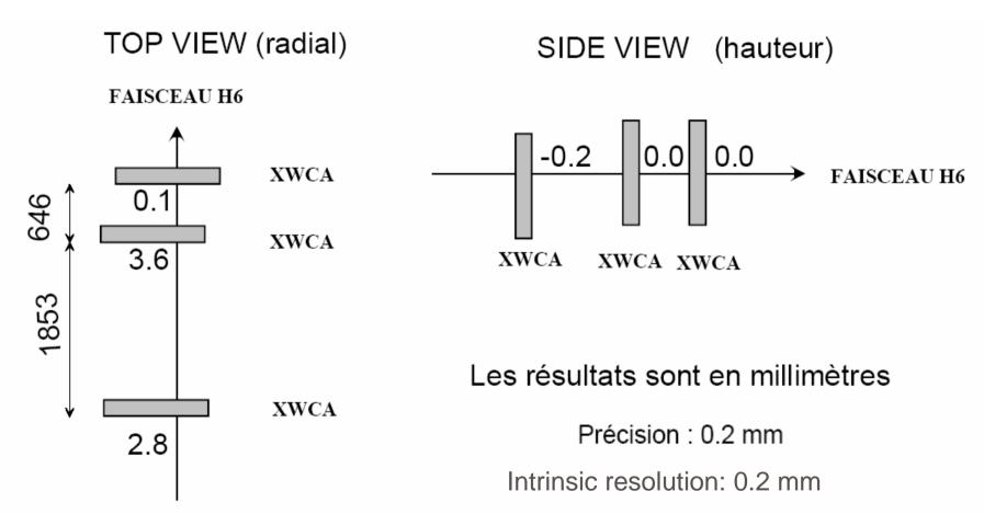
With this good precision, misalignment should not be relevant for tracking resolution
