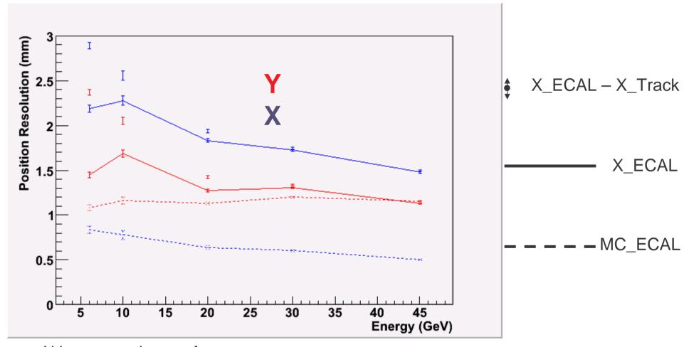
X is centered on wafer Y is centered on gap
