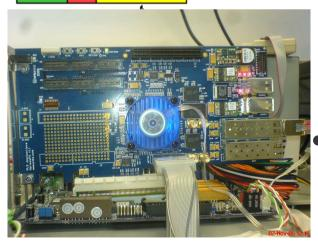
ODR is a commercial FPGA board with PCIe interface
