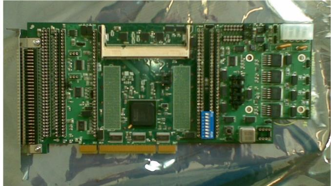
Board has SO-DIMM socket, allowing us to install ram for event buffering.
