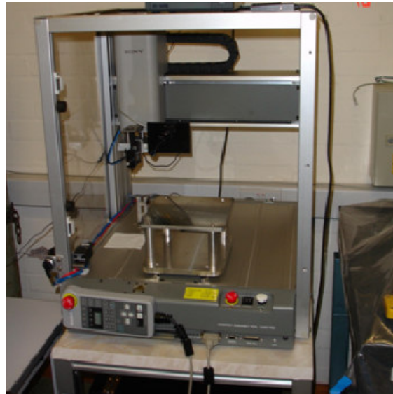
Fig 3 Sony robot with Glue dispenser head
