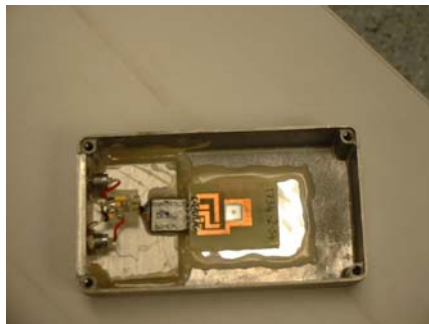
Figure 8 Box (acting as a Faraday cage when covered) for measuring ionising radiation with a silicon detector
