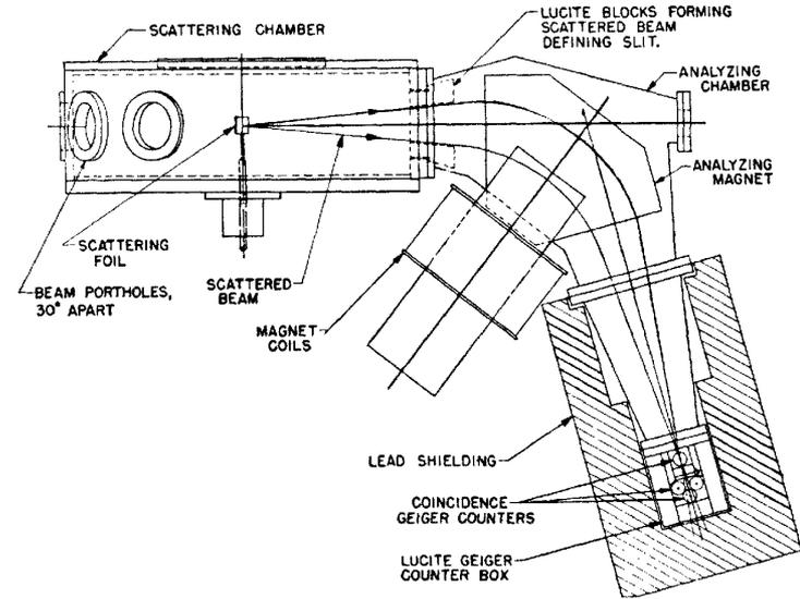
FIG. 2. Scattering chamber.
