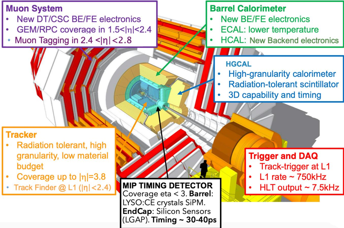
All silicon tracking system with pixels and silicon strips
