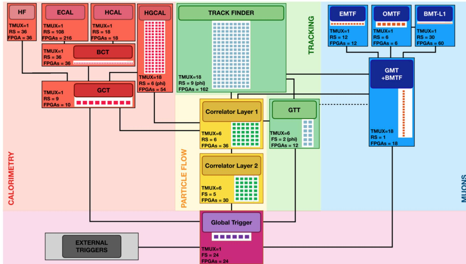
Provides robust independent triggers for **calorimeter**, **muon** and **tracking** systems separately, and a **Particle Flow** trigger, which combines detector information, all feeding into a **global trigger**
