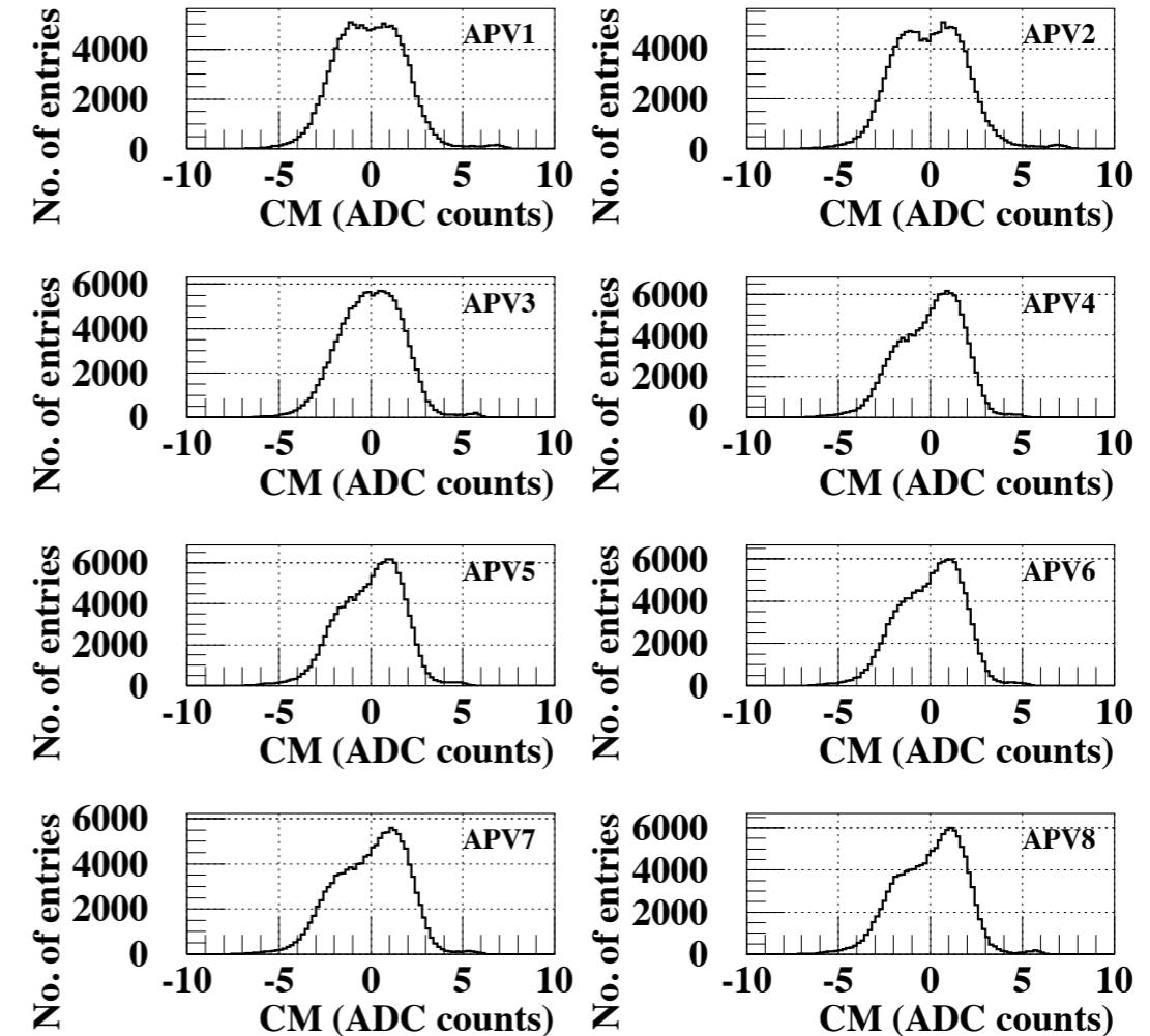
Peaks and drops in noise at end channels not fully understood but very likely from circuit design
